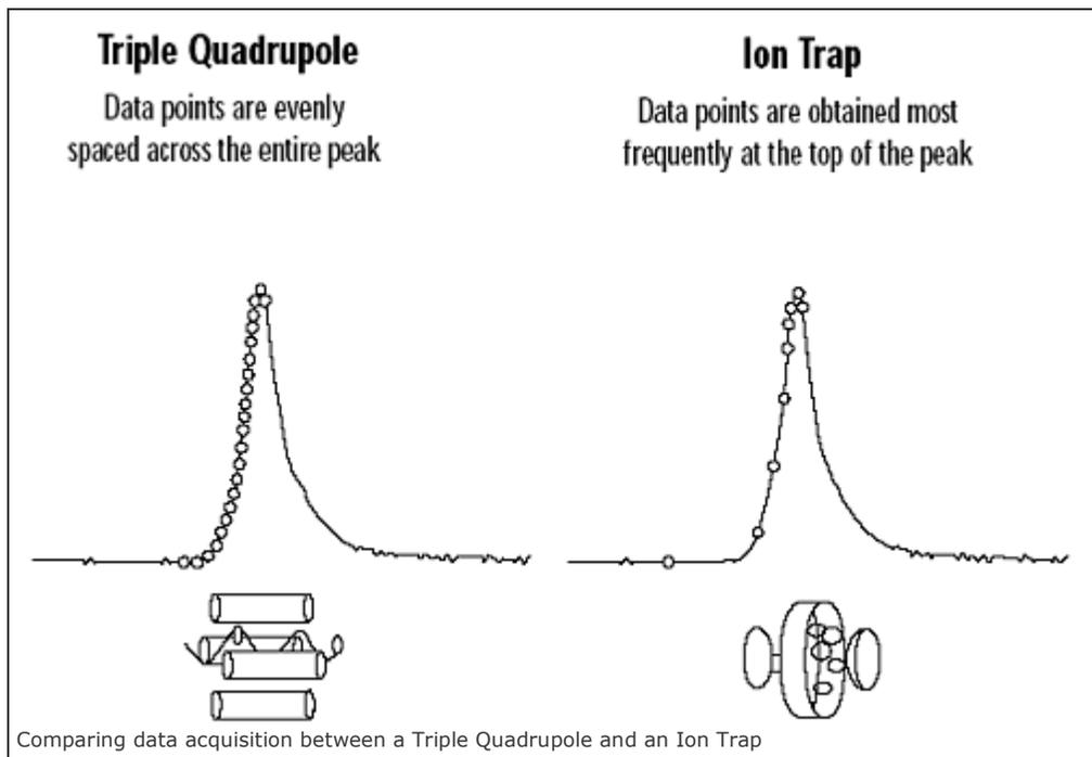
The ion trap is more sensitive in scan mode than in SIM mode.
