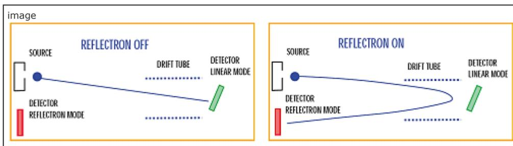
In order to increase the resolution, the ion trajectory is bent by an electronic mirror, the reflectron. When going through the reflectron, the dispersion of ions of the same  $m/z$  value is minimized, leading to a great improvement of resolution
