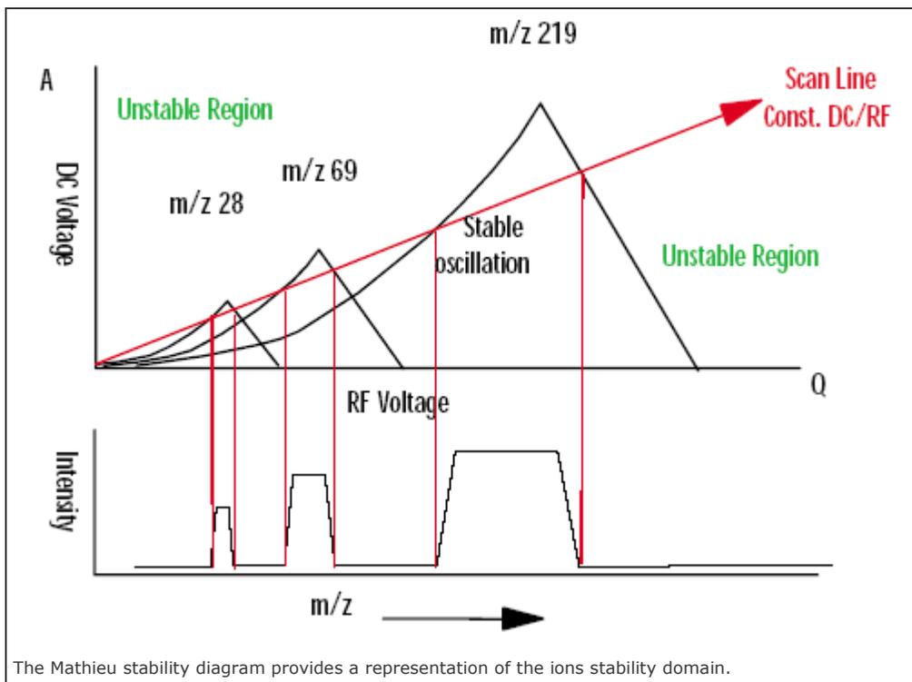
The quadrupole is scanned with  $A/Q = \text{constant}$ ; the resolution depends on the slope of the scan line.
