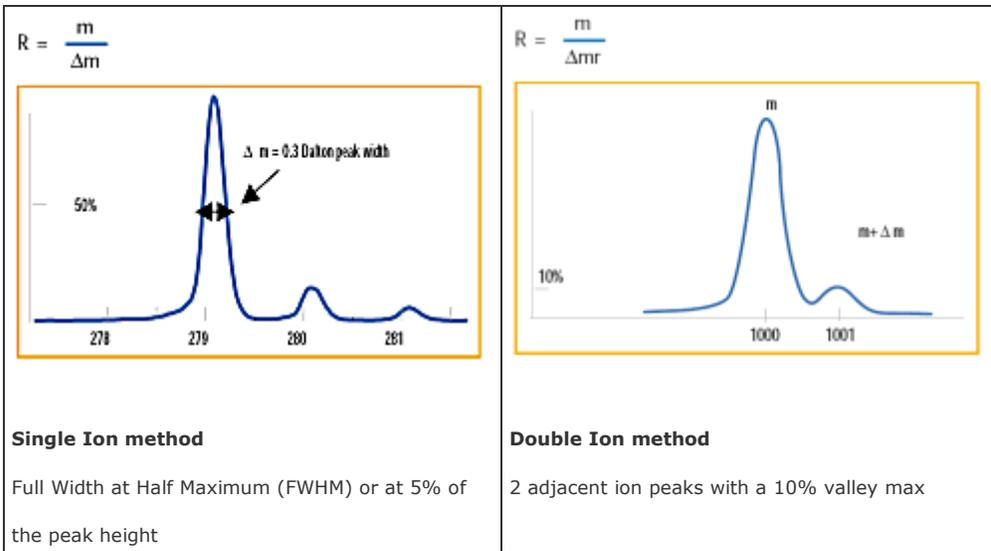
Resolution calculation: the above described methods can be used with various valley and  $\Delta m$  definitions, which are represented on the next figure.
