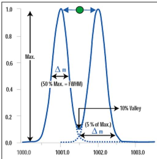
The mass accuracy is the difference which is observed between the theoretical mass and the measured mass:
