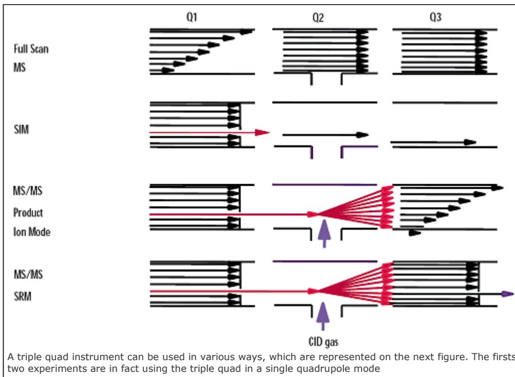
The first quadrupole is used to select a first ion (precursor), which is fragmented in the collision cell. This is typically achieved in the collision cell by accelerating the ions in the presence of a collision gas (argon, helium...).
